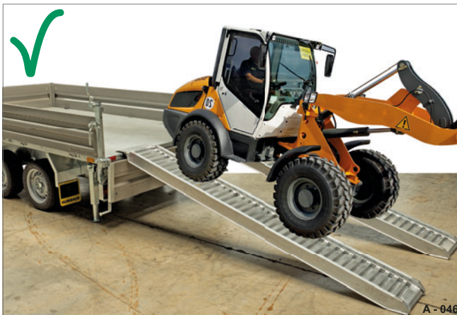
Fig. 101 Driving up the loading ramps
