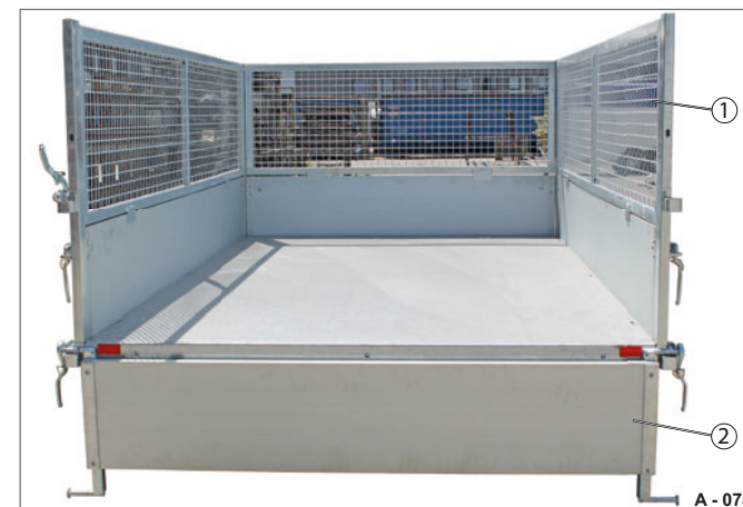
Fig. 58 Rear steel mesh extension removed
