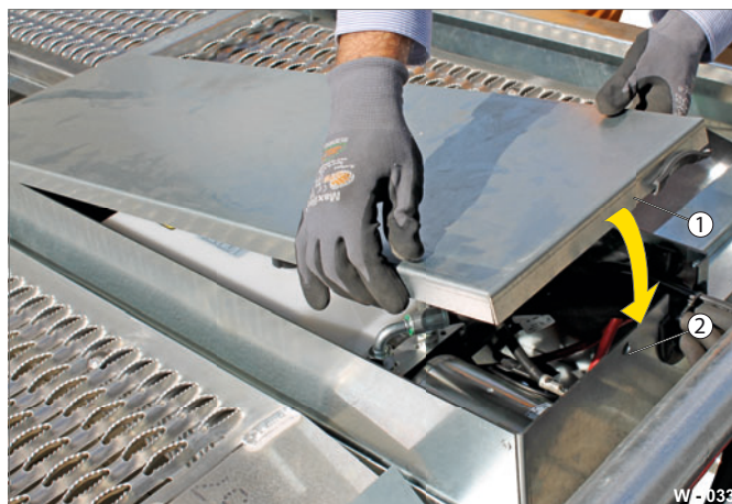
Fig. 27 Installing the supply battery
