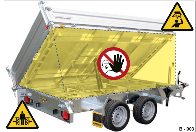
Fig. 7 Tipped at the side / danger areas
