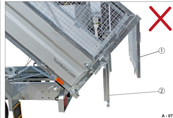
Fig. 46 Steel mesh extension unsecured
