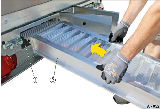
Fig. 106 Inserting the loading ramps
