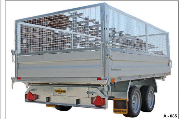
Fig. 67 Steel mesh extension fitted
