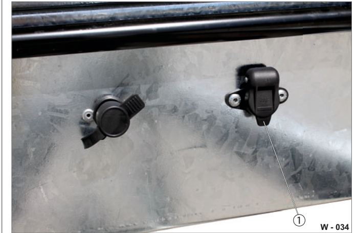
Fig. 30 Connection for battery charging plug
