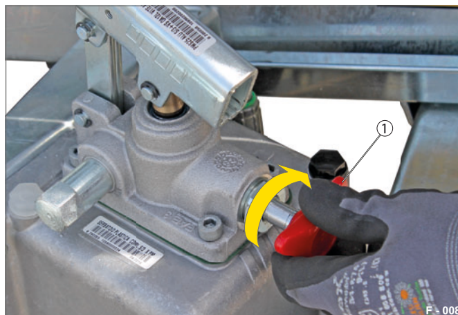
Fig. 2 Close the valve wheel
