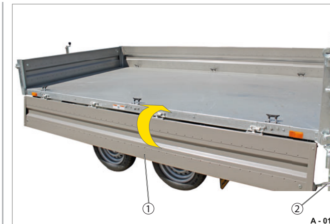
Fig. 16 Close the drop side
