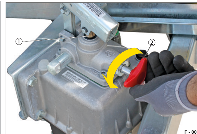
Fig. 9 Close the valve wheel
