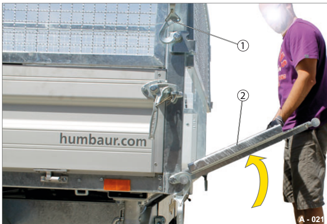
Fig. 20 Close the rear drop side
