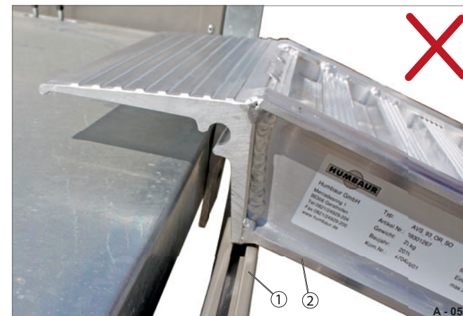
Fig. 97 Loading ramp incorrectly attached
