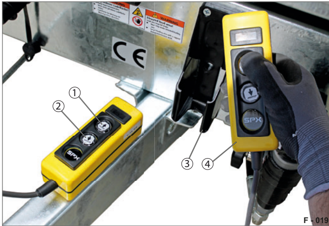
Fig. 17 Tipping the cargo bed
