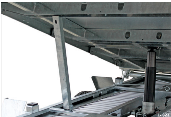
Fig. 25 Maintenance brace for securing the loading bridge
