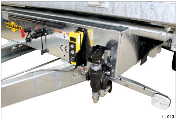
Fig. 24 Hand button and emergency hand pump
