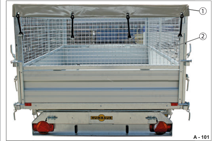
Fig. 80 Flat cover (with steel mesh extension)
