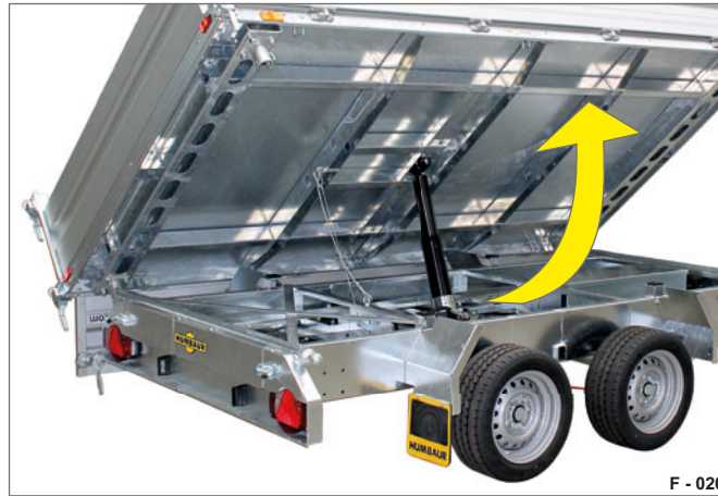
Fig. 18 Tipping the cargo bed
