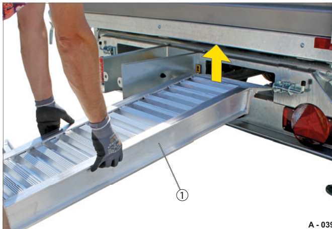
Fig. 90 Lifting out loading ramps
