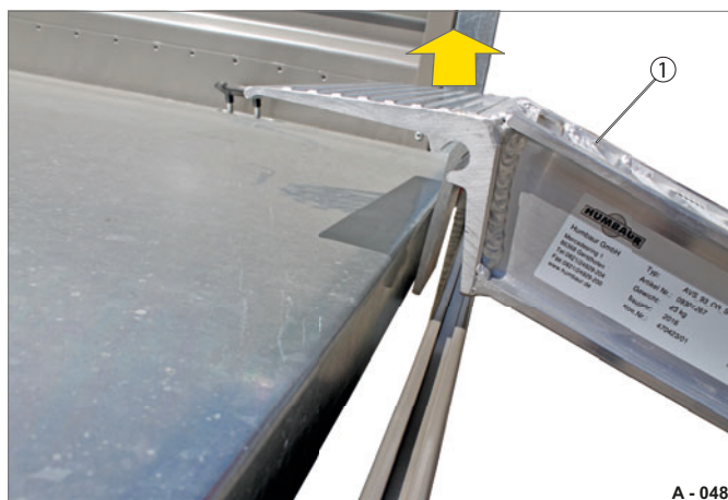
Fig. 103 Lifting the loading ramp
