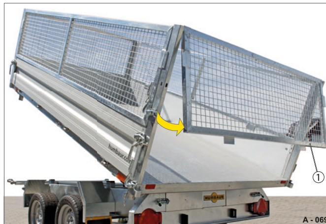
Fig. 45 Steel mesh extension swinging freely
