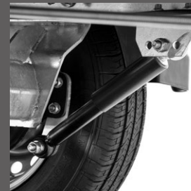
Wheel shock absorbers (mounted) incl. 100 km/h approval*
