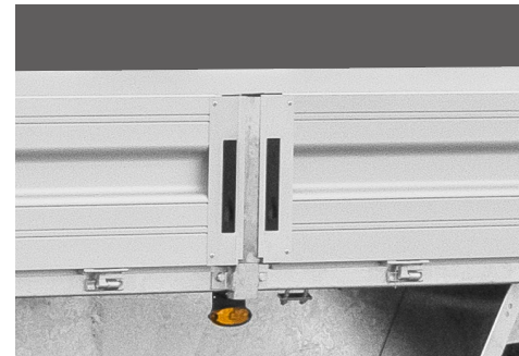
Central stanchions fitted on the divided side plates as standard (from an inner length of 6100 mm)
