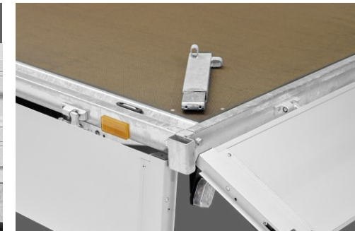
Corner stanchions can be removed when the side plates are lowered
