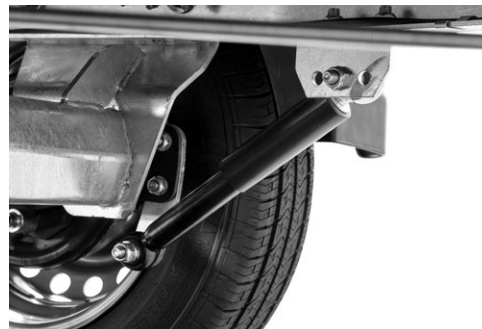
Wheel shock absorber, for 100 km/h version (optional)
