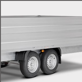
Side plate extension, 350 mm
